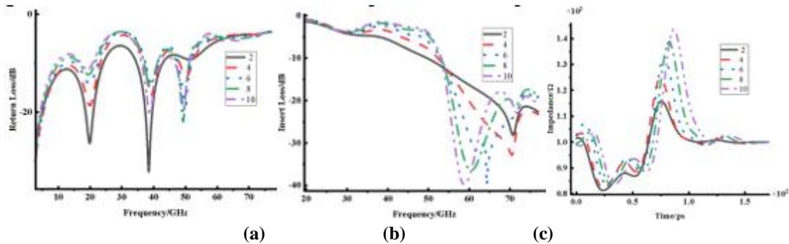
Fig.10 L=30MIL, Effect of the number of reflux perforations on S-parameters and TDR characteristics
