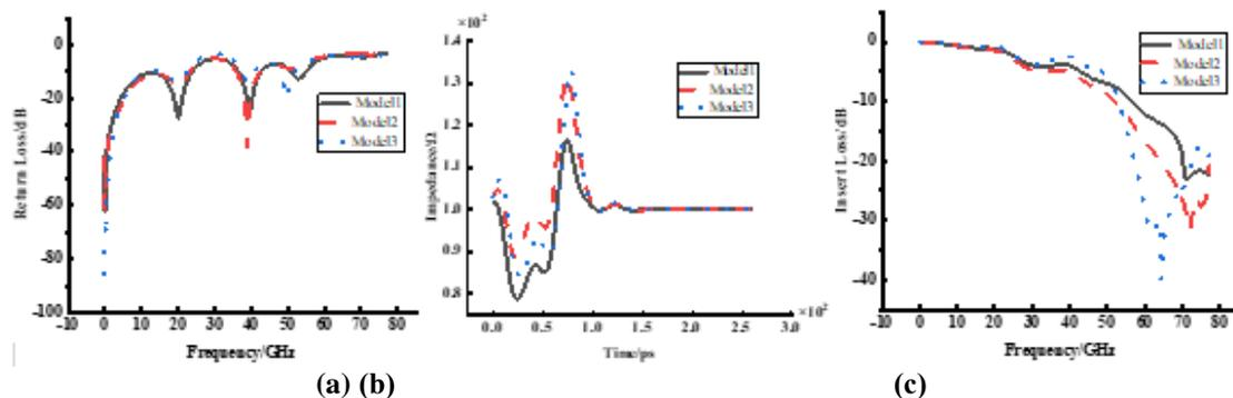
**Fig. 2 S-parameter and TDR waveforms at different locations and numbers of return orifices**
