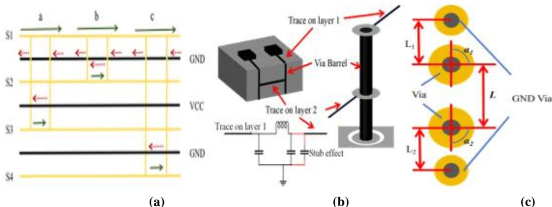
**Fig. 3 (a)Return path of the signal flow through the hole;(b)Equivalent circuit for parasitic capacitance through holes;(c) Differential Line Transition Overhole Structures**
