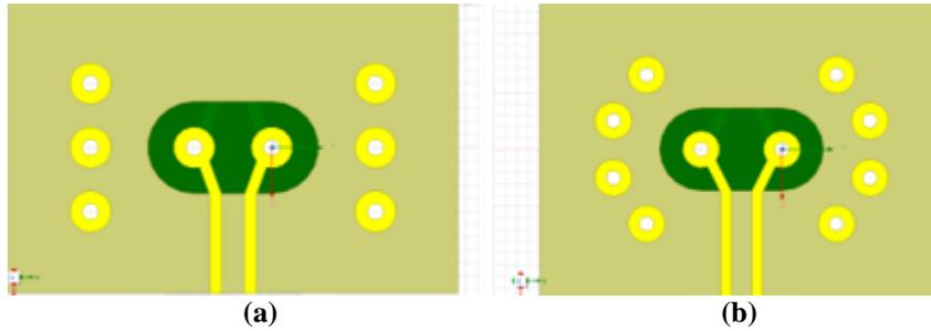
Fig. 8 (a)6 linearly distributed reflux perforation permutation models;(b) Modeling of 8 curvilinear distributions of reflux perforation permutations
