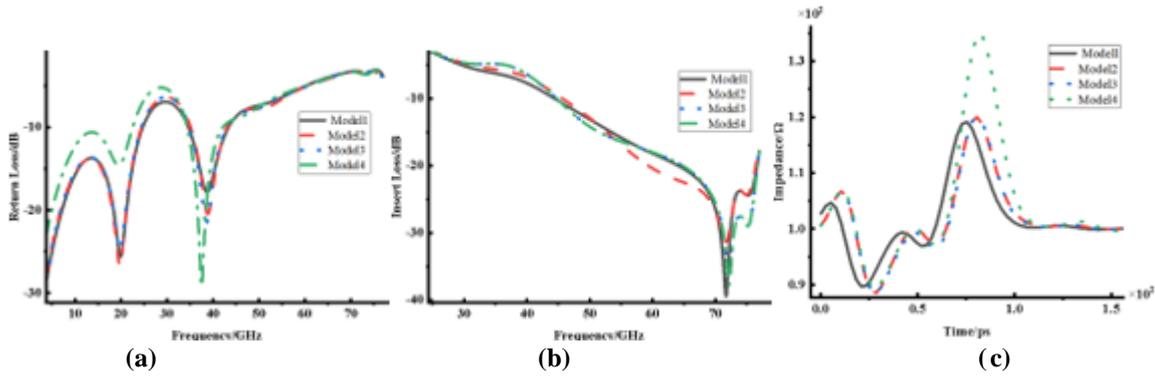
Fig. 6 L1、L2=45mil, (a)Return loss;(b) Insertion loss;(c) TDR waveform
