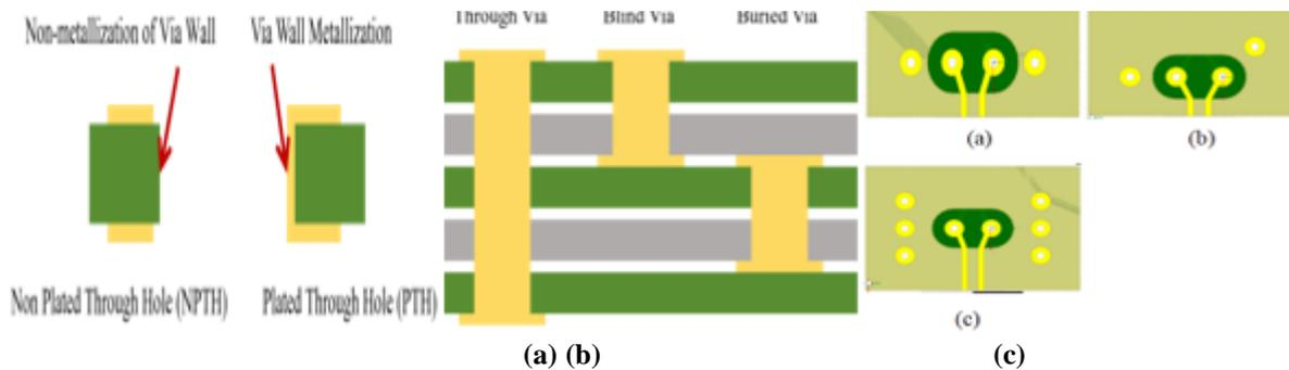
**Fig. 1 (a)Cross-sectional structure of plated holes (PTH,copper thickness $18\mu\text{m}$ ) and non-plated holes (NPTH) (FR4, $\epsilon_r=4.3$ );(b)Classification of perforation production process;(c)3 Models with different locations and number of return orifices**
