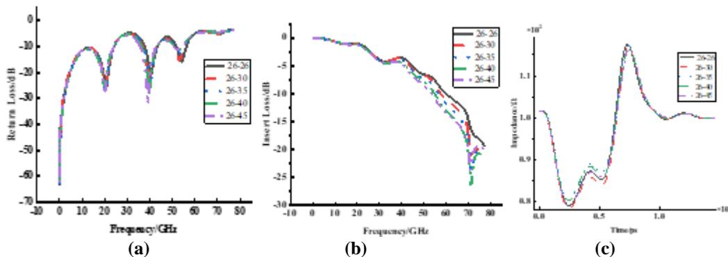
Fig. 7When L=30mil and L1≠L2 (a)Return loss;(b) Insertion loss;(c) TDR waveform
