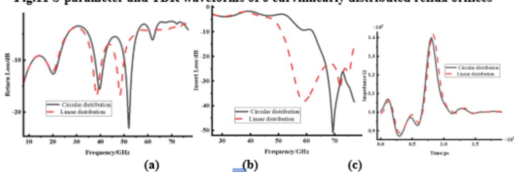
**Fig.12 S-parameter and TDR waveforms of 8 curvilinearly distributed reflux orifices**
