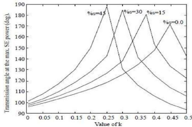
Fig 9. Variation in transmission angle at the max. SE power for diff. %S
