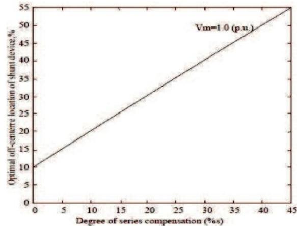
Fig 11. Variation in the optimal off-center location of shunt FACTS device against degree of compensation of line (%S).
