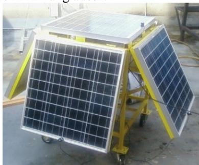
Figure 3: Orientation of PV modules at 4 different slopes [9].
