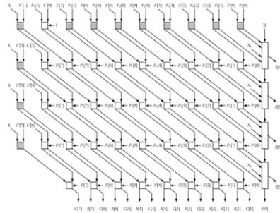
Figure 8 Architecture of the Proposed CSA tree
