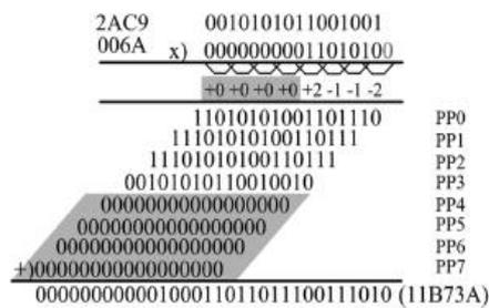
Figure 2 Illustration of multiplication using modified FIR encoding
