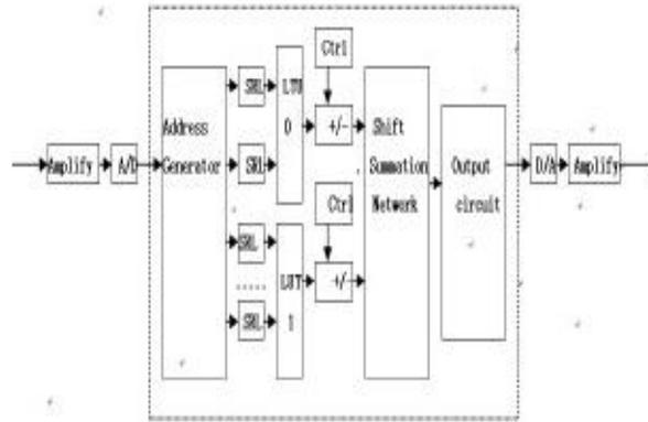
Figure 10 The circuit structure of FIR system
