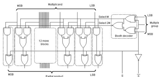
Figure 3 FIR partial product selector logic
