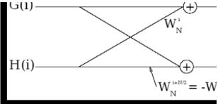
Fig 2: Basic butterfly computation in the decimation-in-time FFT algorithm.
