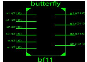
RTL View Of A Butterfly Component Used In 32-Point FFT
