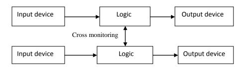
Fig. 7: Category 4 safety block diagram with cross monitoring logic
