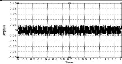
Figure 3: Vibration signal of Healthy Bearing.
