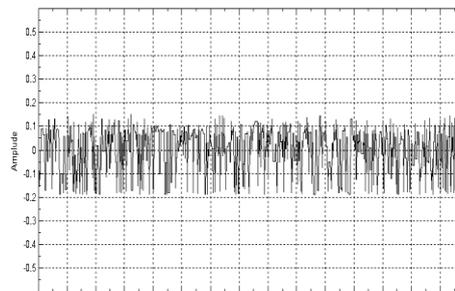
Figure 5: Vibration Signal of bearing with inner raceway defect
