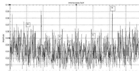
Figure 6: Frequency Spectrum for bearing with inner raceway defect.
