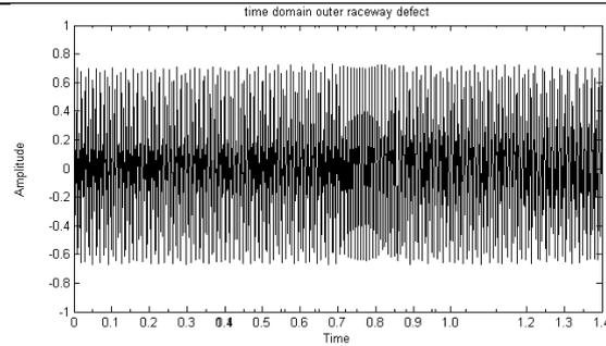
Figure 7: Vibration Signal for bearing with outer raceway defect.
