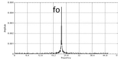
Figure 4: Frequency Spectrum for healthy bearing.
