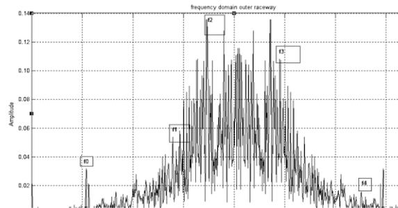
Figure 8: Frequency Spectrum for bearing with outer raceway defect.
