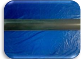
Fig.(2) The halved PVC pipe.
