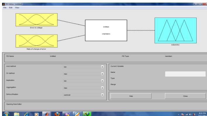
Here are 2 inputs and one output in the structure as shown in FIS editor. The next thing to be done is defining the membership functions for all the input and output variables. This will be done in the membership editor as shown.
