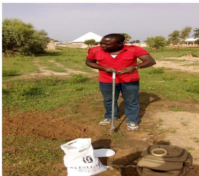
**Plate 4.4: using spiral auguring for Soil data collection during Field Work**
