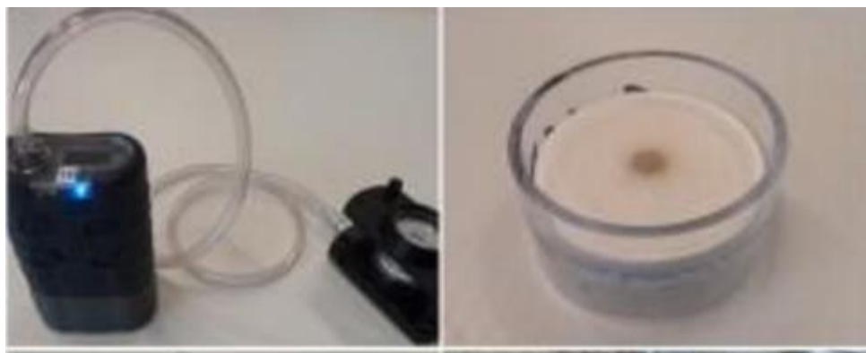
Figure 3: Sampling equipment (pump and cassette)
