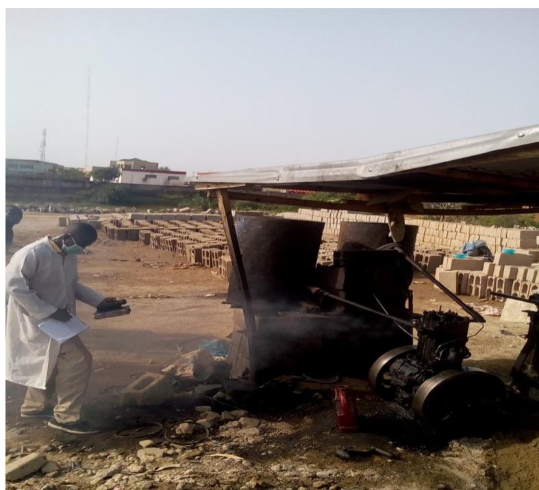
Fig. 2: 12 Hp water-cooled Diesel Engine during Monitoring
