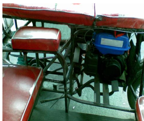
Figure 1. (a) The motorized pedicabs or "kuliglign". (b) The engine of a "kuliglign" plying the major roads of Manila.
