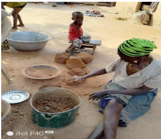
Plate 3: Kuku community potter mixing grog with plastic clay
