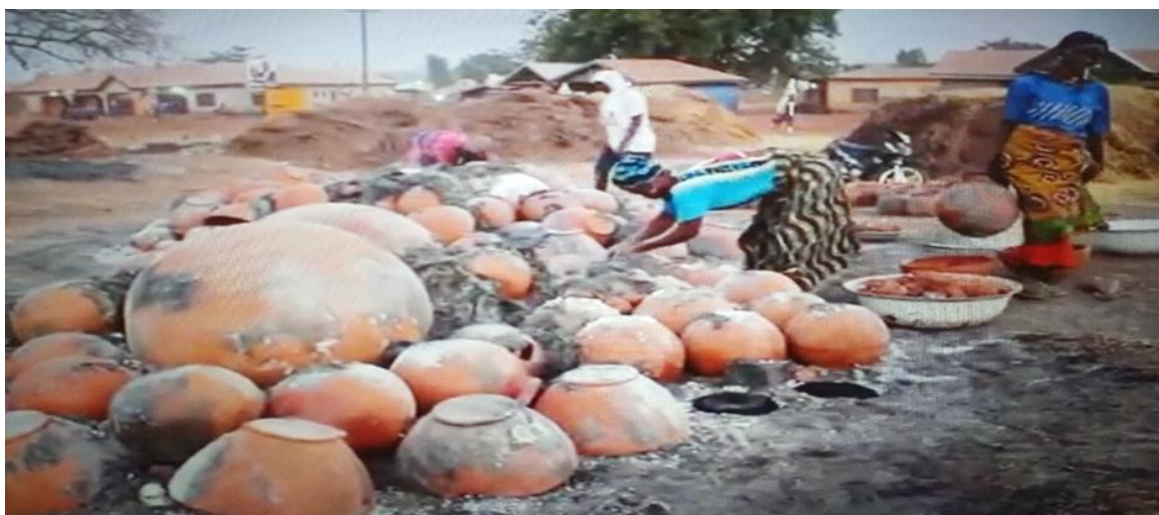
Plate 15: Pottery pieces are left to cool gradually within the embers
