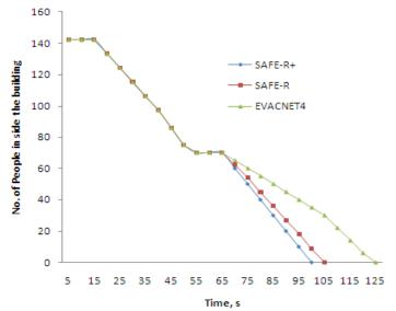
Table 5 shows the activated paths, which have been used by the evacuees to evacuate the building. The actual evacuation process started only after 15s this is due to the activation time of the paths 1, 3,6,11. The path 4 activates after 30s and starts the evacuation process.
