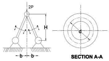
Fig. 4.Two bar truss under load
