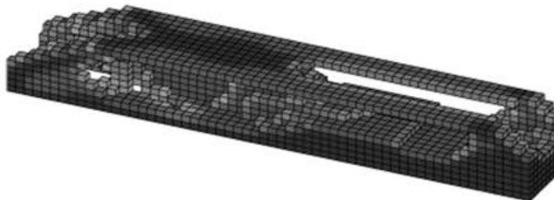
Fig -2: Topology optimization of MBB-Beam (Matlab)
