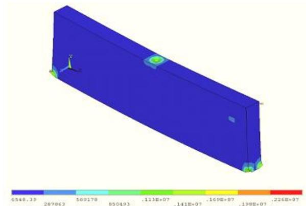
Fig -6: Von Mises stress plot
