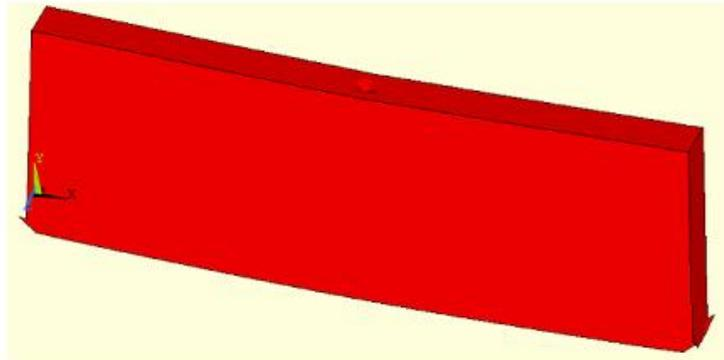
Fig -3: Initial structure (MBB-Beam)
