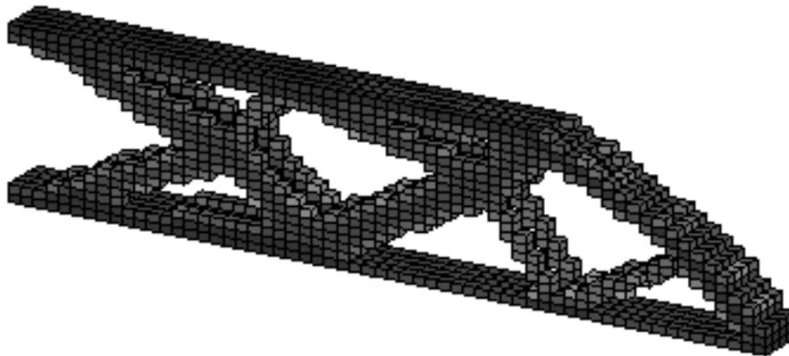
Fig -9: Topology optimization of Cantilever-Beam (MATLAB)
