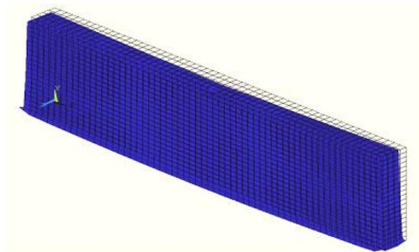
Fig -5: Displacement plot with deformed structure
