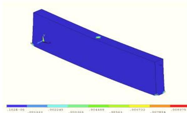
Fig -7: Von Mises elastic strain plot
