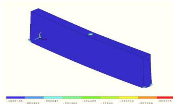
Fig -7: Von Mises elastic strain plot
