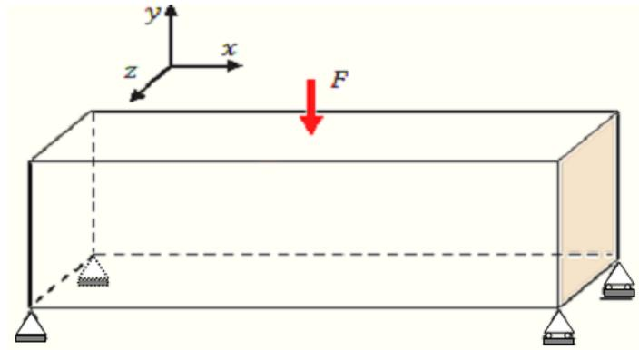
Fig -1: MBB Beam with boundary conditions and loads
