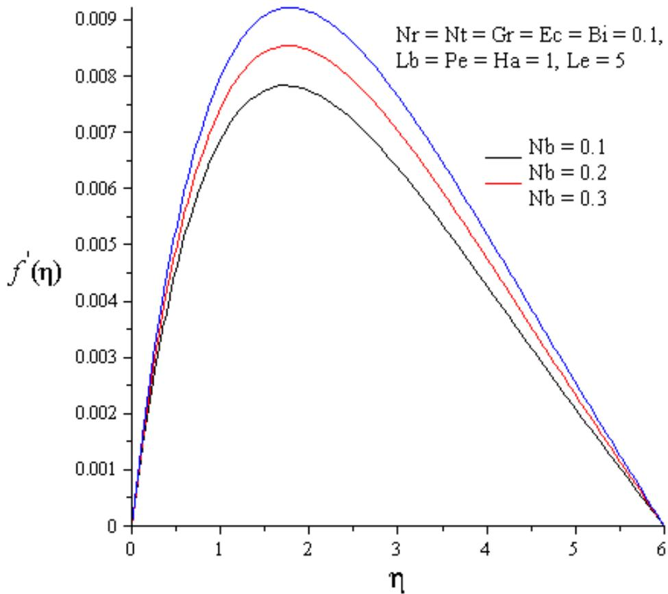
Figure 5.4: Effects of Brownian motion on velocity
