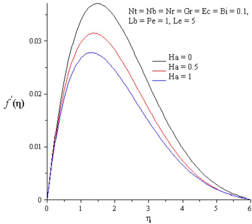
Figure 5.1: Effects of Hartman number on velocity
