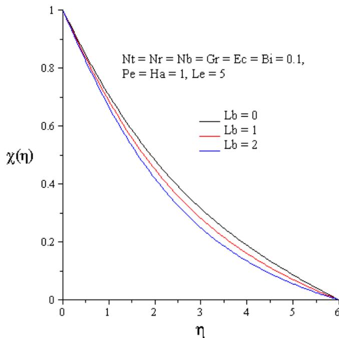
Figure 5.14: Effects of bioconvection lewis number on microorganism concentration
