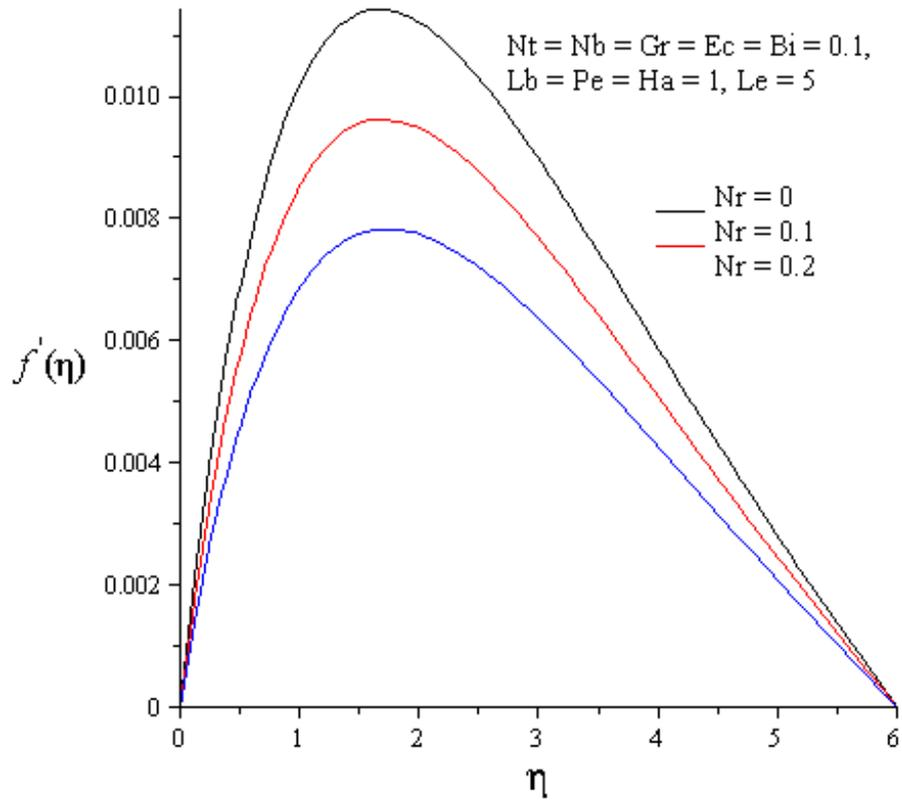
Figure 5.3: Effects of buoyancy ratio on velocity
