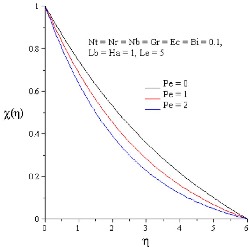
Figure 5.15: Effects of bioconvection pecelet number on microorganism concentration
