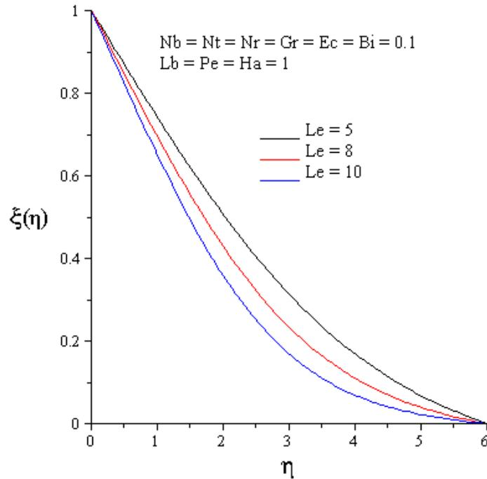
Figure 5.13: Effects of traditional lewis number on nanoparticle concentration
