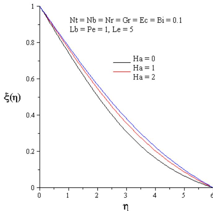
Figure 5.10: Effects of Hartman number on nanoparticle concentration
