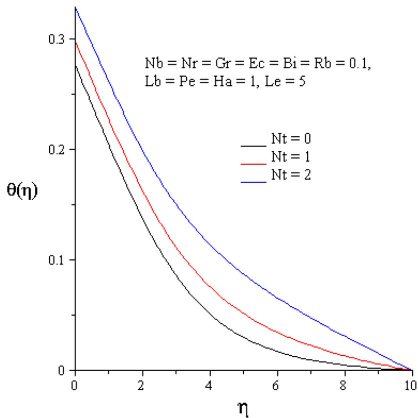
Figure 5.8: Effects of Thermophoresis on Temperature
