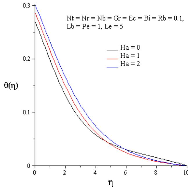
Fig 5.6: Effects of Hartman number on Temperature
