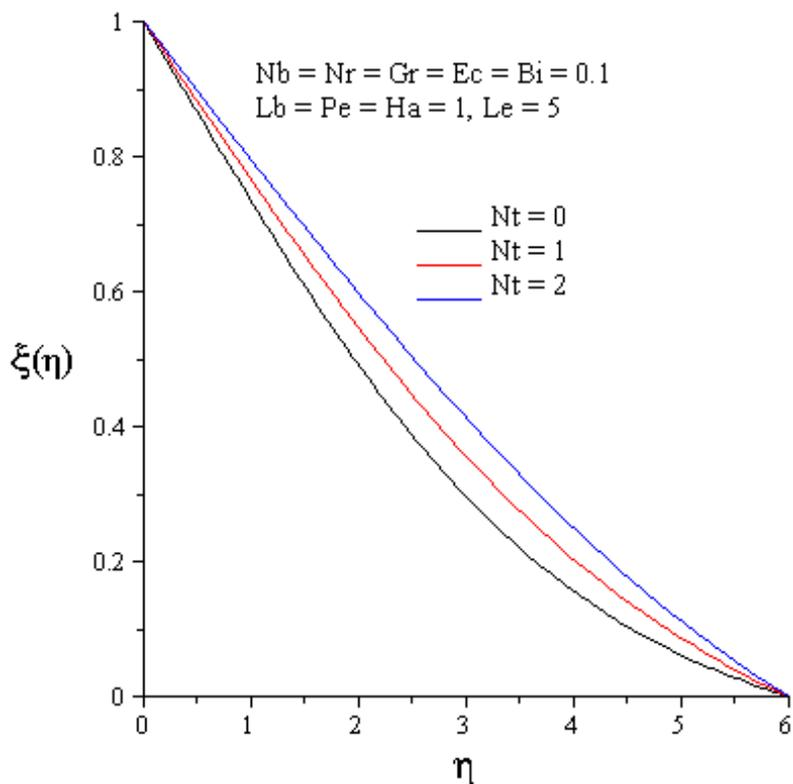
Figure 5.11: Effects of thermophoresis on nanoparticle concentration
