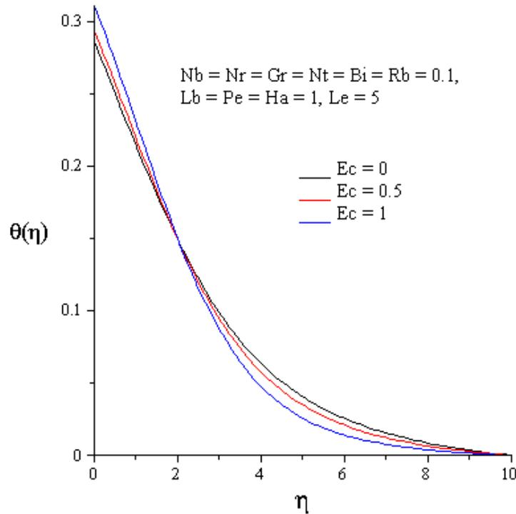
Figure 5.9: Effects of Eckert number on Temperature
