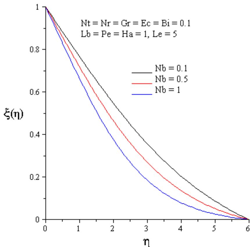
Figure 5.12: Effects of Brownian motion on nanoparticle concentration
