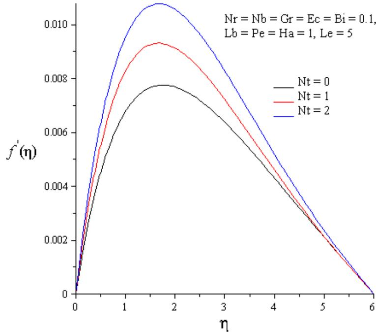
Figure 5.5: Effects of thermophoresis on velocity
