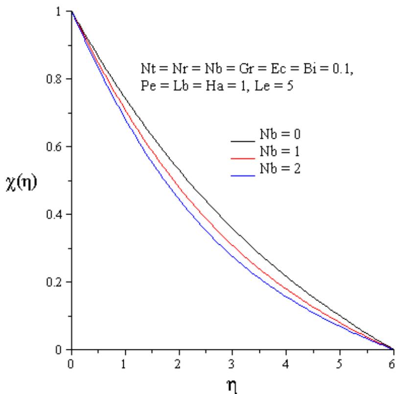
Figure 5.16: Effects of Brownian motion on microorganism concentration
