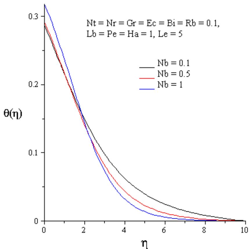
Fig 5.7: Effects of Brownian motion on Temperature
