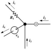
Referring to the diagram above, the current entering any junction is equal to the current leaving that junction. Hence,  $i_1 + i_4 = i_2 + i_3$
