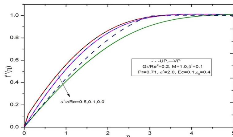
**Fig.6.** Velocity profiles for different values of  $\alpha^*/\sigma Re$  for UP and VP
