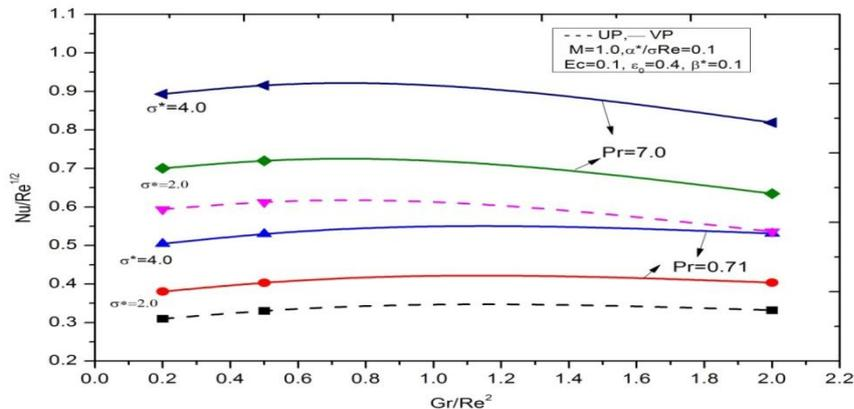
**Fig.2.** Nusselt number for various  $Gr/Re^2$ ,  $\sigma^*$  and Pr for UP and VP
