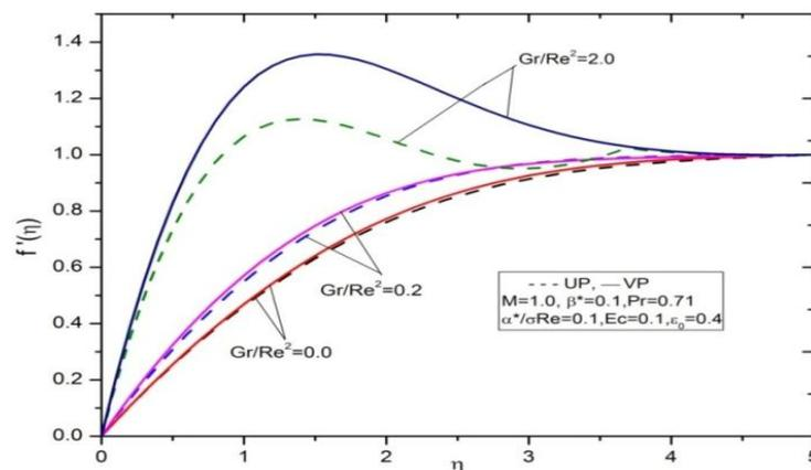
**Fig.5.** Velocity profiles for different values of  $Gr/Re^2$  for UP and VP
