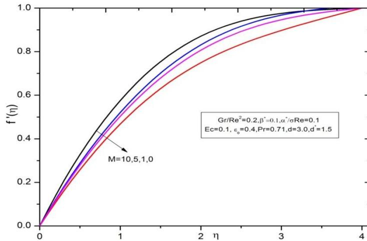
**Fig. 3.** Velocity profiles for different values of M for VP
