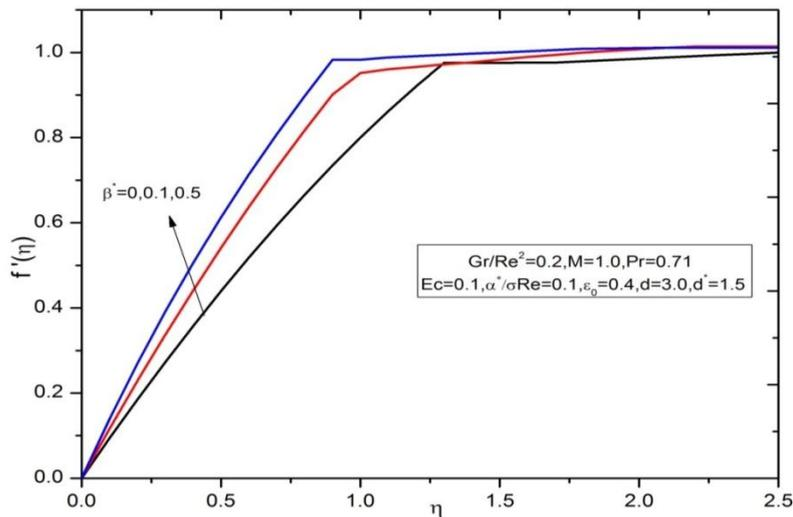
**Fig.4.** Velocity profiles for different values of  $\beta^*$  for VP
