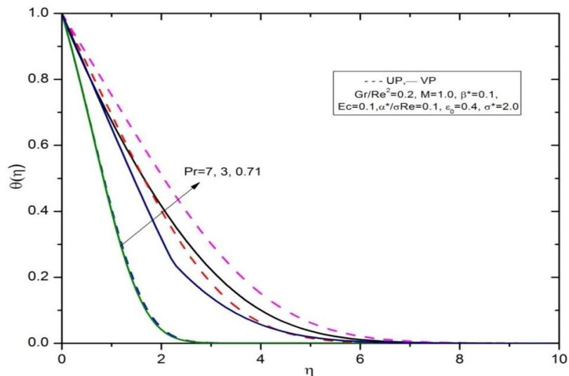
Fig. 13. Temperature profiles for various values of Pr for VP
