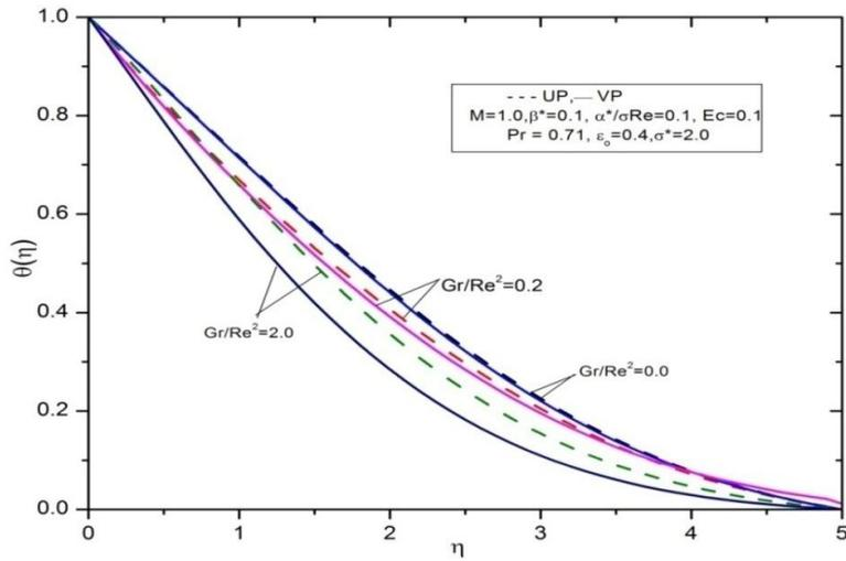
Fig.10. Temperature profiles for various values of  $Gr/Re^2$  for UP and VP
