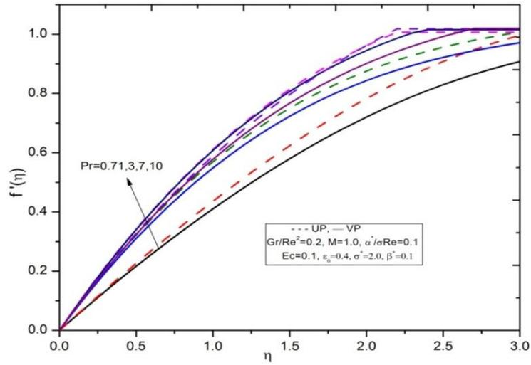
Fig.7. Velocity profiles for different values of Pr for VP
