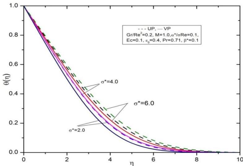
Fig. 12. Temperature profiles for various values of  $\sigma^*$  for UP and VP
