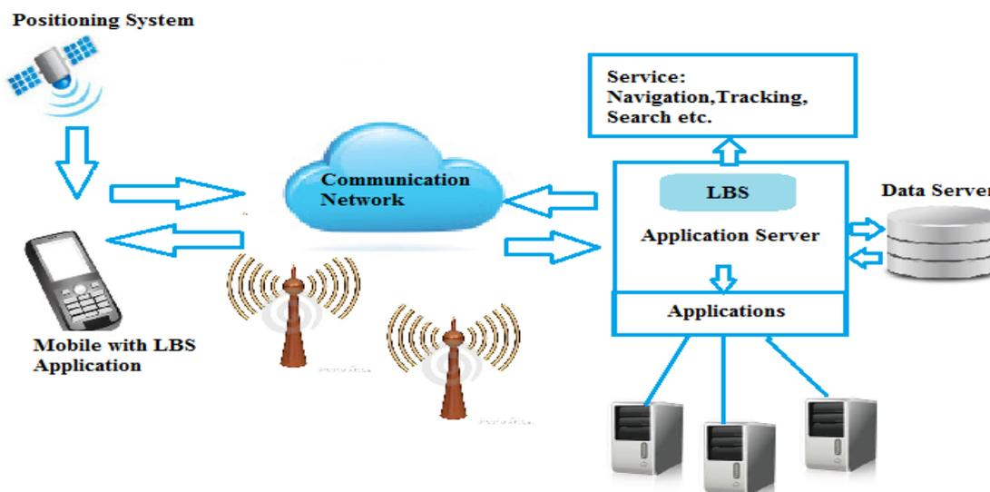
**Fig 1. LBS Architecture showing various elements of the Communication Model.**
