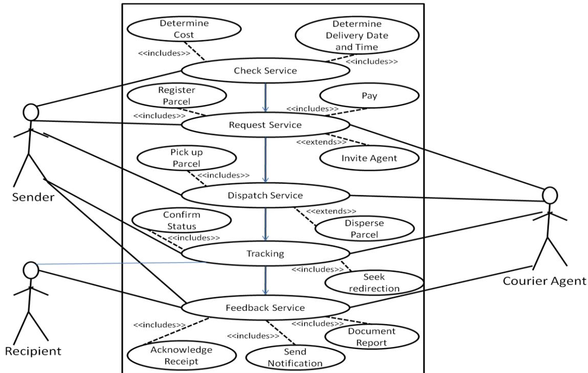
Figure 1: UML use case diagram for the interactive mobile courier system
