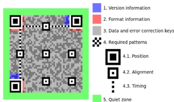
Fig 2: Structure example of QR code
