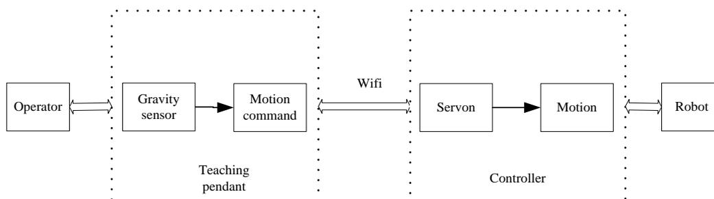
Fig.1 The teaching pendant process of the robot
