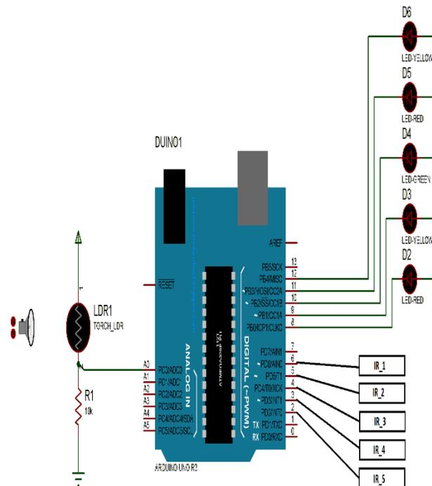
Fig. 4.1. Block diagram for Smart street light using IR sensors
