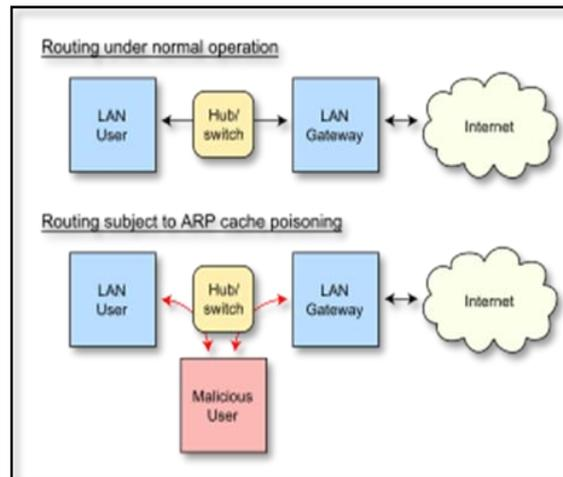
Fig. 2 ARC Cache Poisoning
