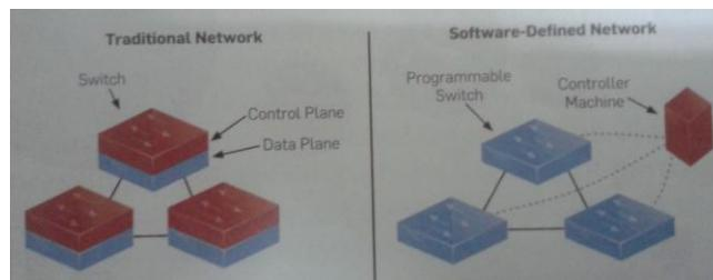
**Figure 1.** Traditional and Software-Defined Architectures
