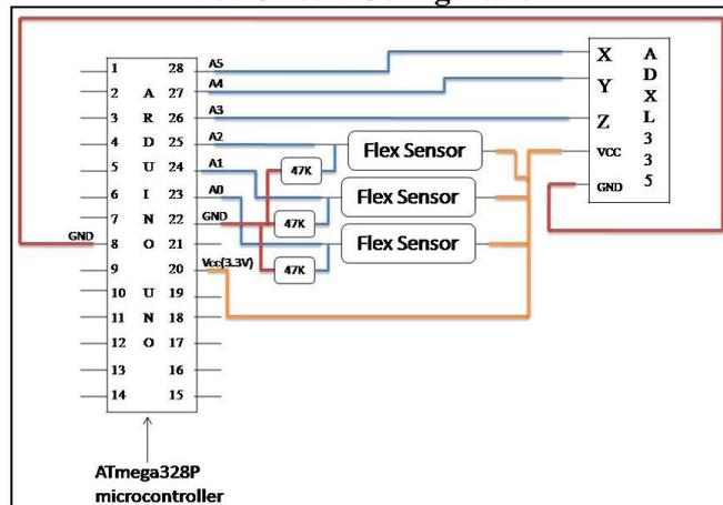
Fig 2.: Circuit Diagram of VR Glove
