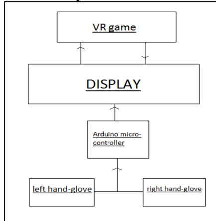
Fig 1.: Block Diagram of VR Glove
