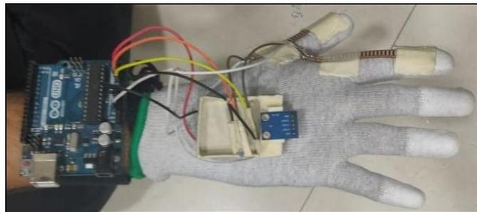
Fig 4.: Construction of the first Prototype of VR Glove
