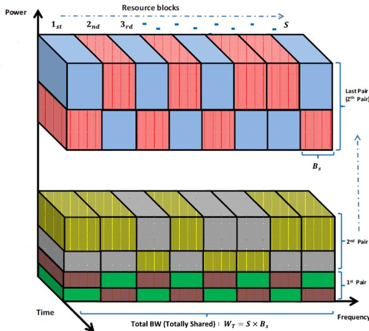
**Fig 3 : NOMA structure with vertical pairing concept [2]**
