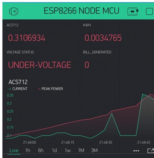
ACS712 connected to A0 pin of Node MCU. Bulb connected to ACS712 and Voltage regulator. Regulator is to vary the voltage intake. This will allow to tell if incoming voltage is low, medium or high. To analyse the reading, we'll use Blynk IoT platform. Blynk is a mobile application that allows to connect to our hardware over internet. This will also allow us to control the hardware from the Blynk mobile application. We can also grab the readings from the sensor to our mobile application.
