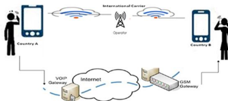
Fig 3. A unified Model of Bypass Structure
