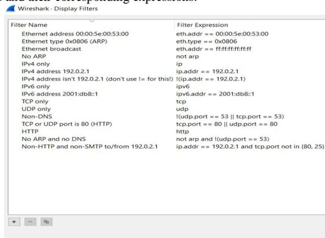
Fig.6: Filters that may be applied in Wireshark to independently monitor network traffic of interest
