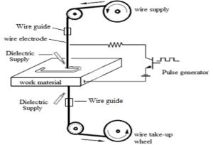
Fig. 1 Wire Electrical Discharge Machining (WEDM) process [12]
