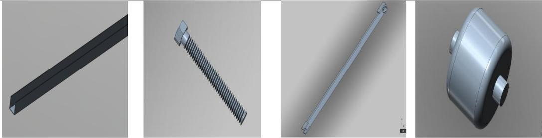
Fig. 3 Cross guide rail, screw, sponge holder, sliding roller for blackboard Erasing machine mechanism
