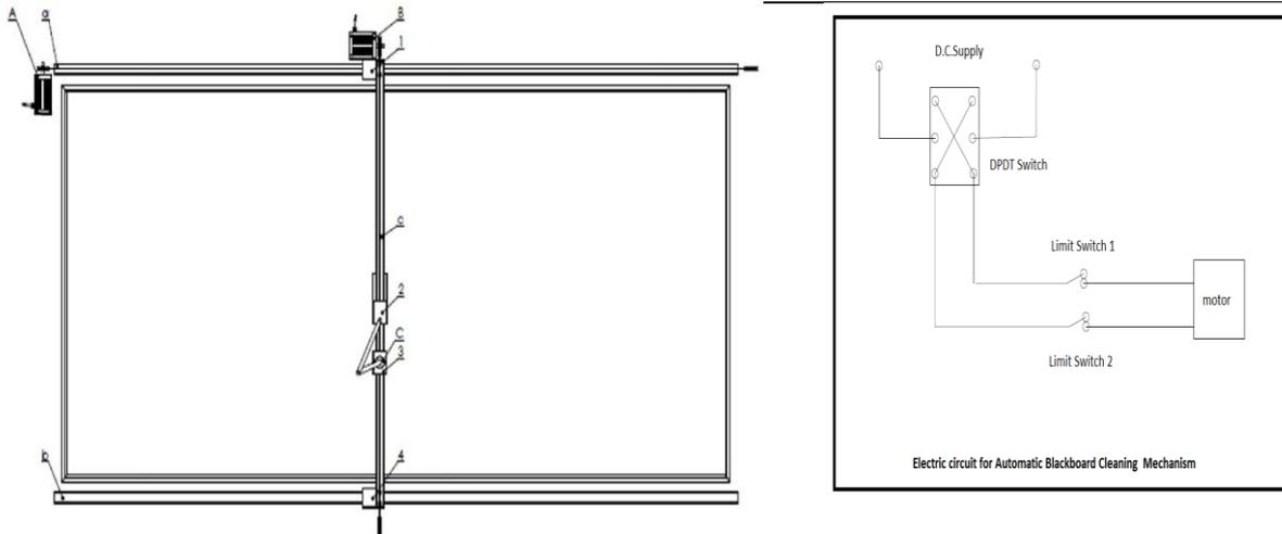
A-Motor for horizontal sliding of cross guide rail C, B- Motor for Vertical sliding wipe system
