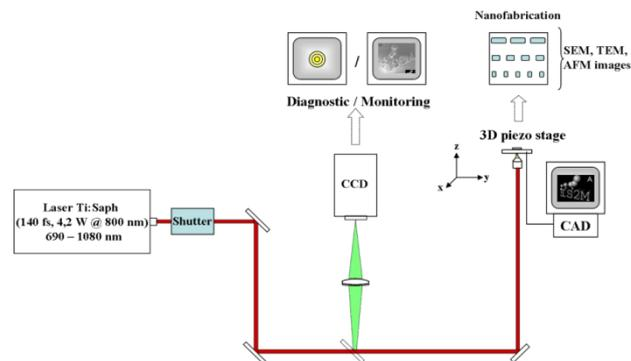
Figure 2 Experimental Setup of a Two Photon Stereolithography Process <sup>[9]</sup>
