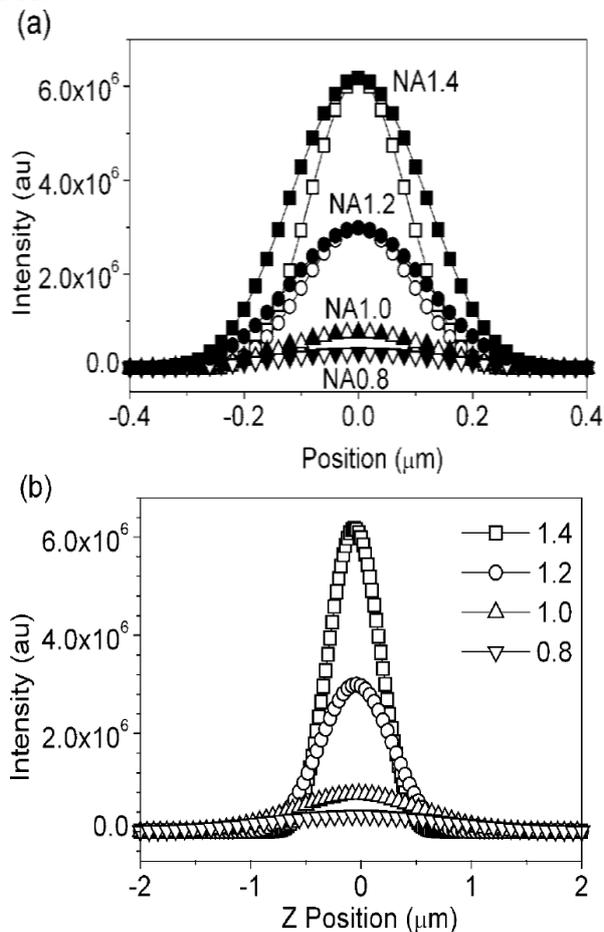
Figure 3 Theoretical two-photon point spread function of different NA focusing calculated using vectorial Debye method<sup>[14]</sup>
