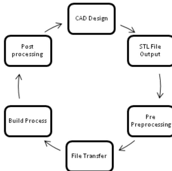
Figure 1 The Rapid Prototyping Cycle <sup>[5]</sup>
