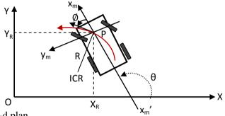
Fig.1 robot model in 2-d plan
