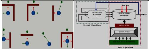
Fig. 3 (a) various situation of obstacle avoidance (b) architecture of the control algorithm for erection of navigation strategies
