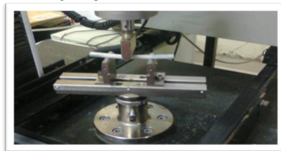
Fig. 12 During flexural test
