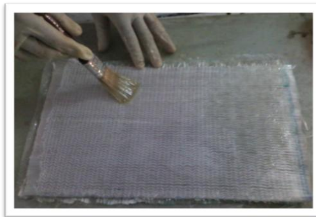
Fig. 7 Applying epoxy resin on fiber
