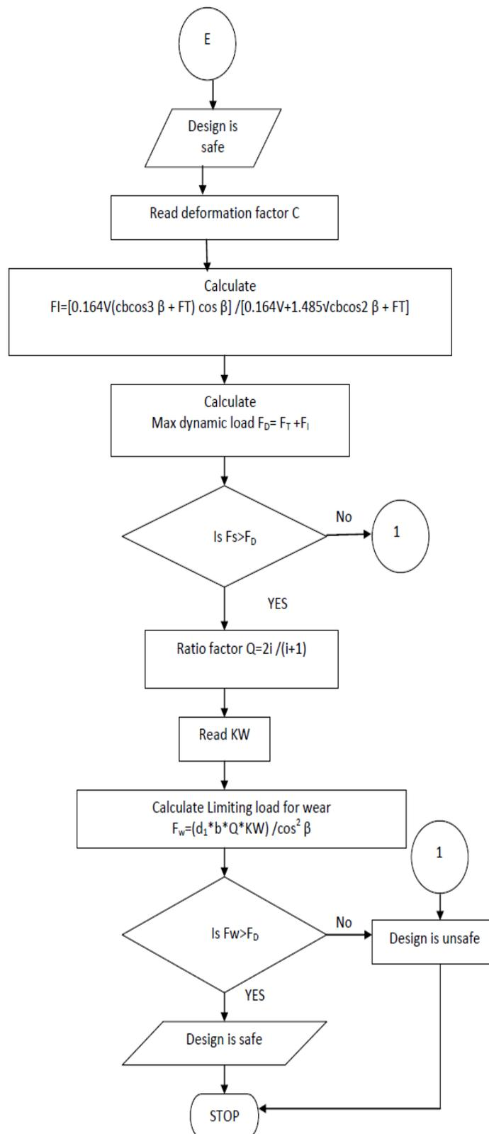
Fig.1. Flow chart for the process of helical gear design.
