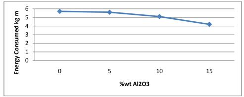
Fig:3.4.1Impact load absorption(In kg m) with % wt Al2O3
