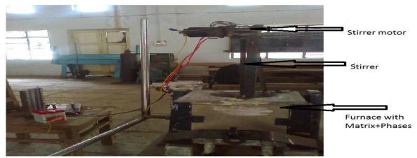
Fig 2.1.3 Induction furnace with stirrer mechanism
