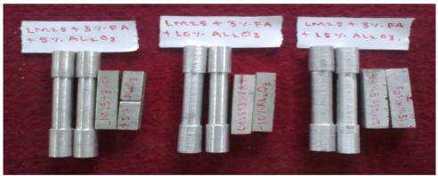
Fig 2.1.5 Tensile and impact test specimen with varying composition of Al2O3
