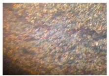
Image 3b.Micro structure of LM25 with 10% Al2O3 and 3% Flyash
