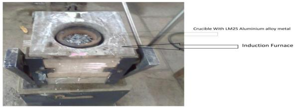
Fig.2.1.1 Induction furnace with Crucible containing LM25
