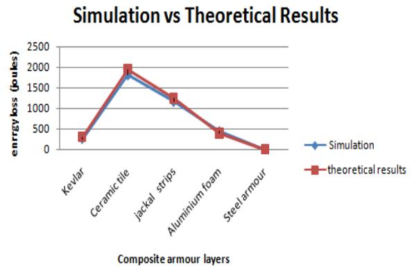
**Fig 14: Simulation vs Theoretical modeling- Energy loss of projectile**
