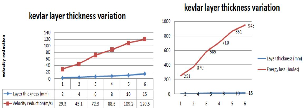
**Fig 18: Graph of velocity reduction in projectile Fig 19: Graph of Energy loss in projectile**
