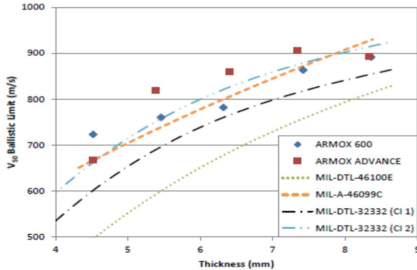
**Fig 1: Ballistic performance will generally increase with hardness, this will depend on the threat projectile and armor thickness and toughness.[6]**
