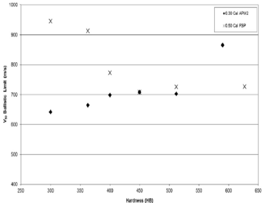
**Fig 2: In the fully hardened condition, with hardness between 510 and 710HV, all targets suffered from gross cracking, whereas when tempered back to 380HV, the tool steels.[6]**
