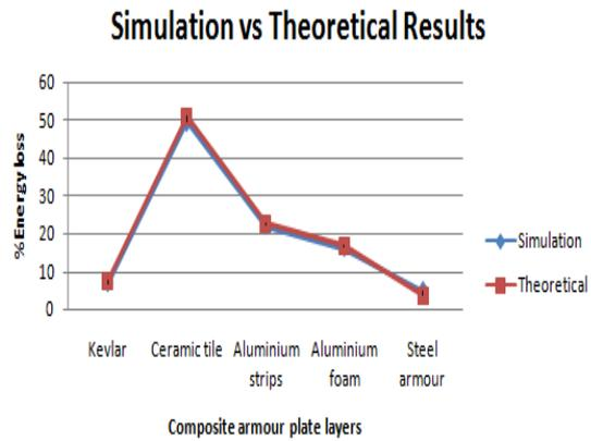
Fig 9: Energy loss of projectile Fig 10: Simulation vs Theoretical modeling- %Energy loss of projectile
