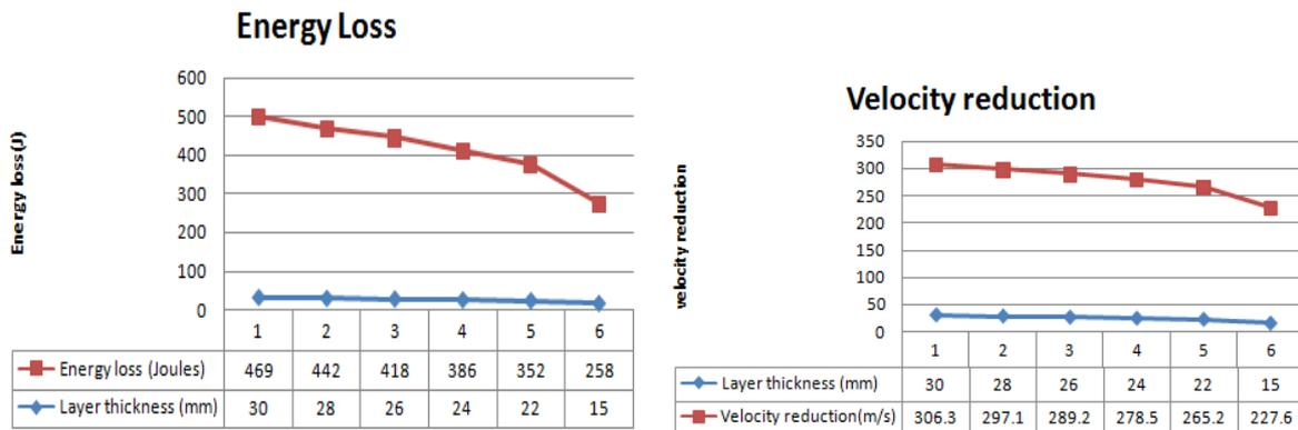
**Fig 20: Graph of Energy loss in projectile Fig 21: Graph of velocity reduction in projectile**
