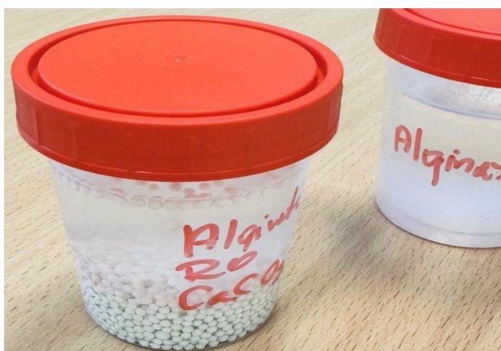
Figure 1. Healing agent for concrete with micro-balls of sodium alginate (by author Isaac Odiri Agbmu)
