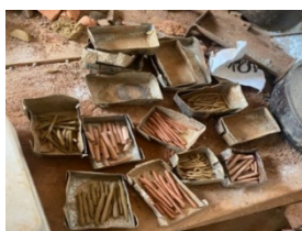
Plate 5: Dried Clay Samples after undergoing Shrinkage limit Plasticity Test
