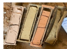
Plate 6: Clay Samples after undergoing Shrinkage limit Plasticity Test
