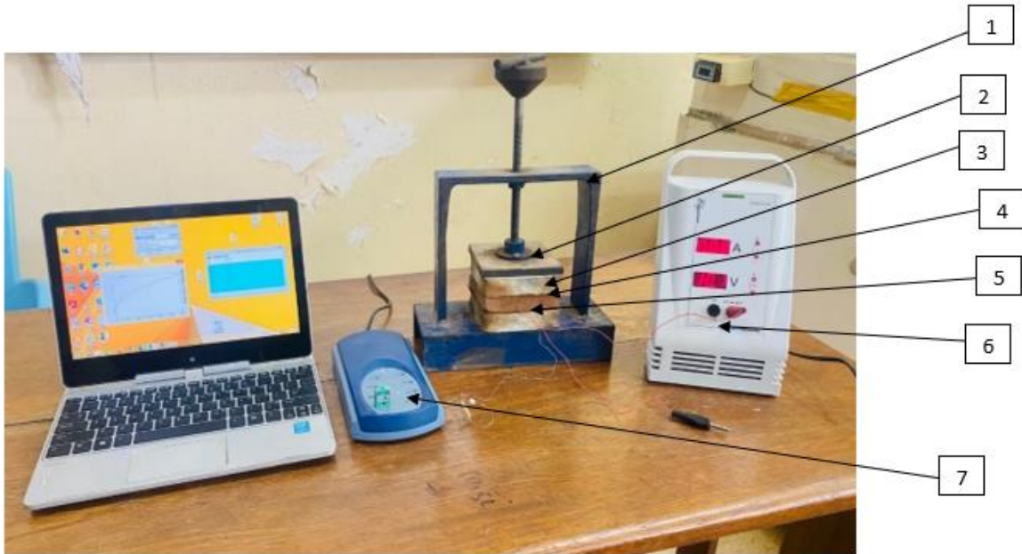
1- Hoist (frame), 2-Clamping device, 3-Sample, 4-Heating resistor, 5-Insulators, 6- Stabilized power supply, 7- Temperature recorder.
