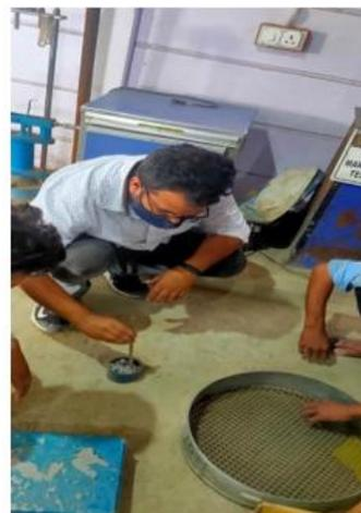
**Fig3.3-Tamping on Aggregates**
