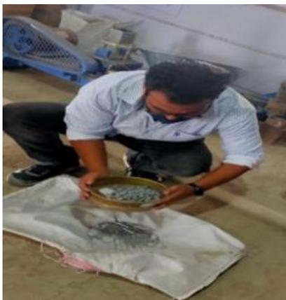
**Fig3.4- Sieve with 2.36mm Sieve**
