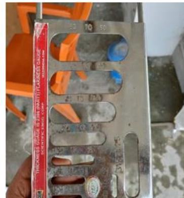
**Fig3.7-Aggregates passing through F. G      Fig3.8-Flakiness Gauge**
