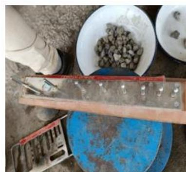
**Fig3.9-Passing aggregates by Elongation gauge      Fig3.10-Elongation Gauge**
