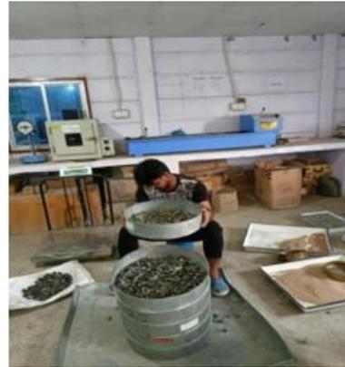
**Fig3.6- Sieve Used in Flakiness and Elongation Indices**
