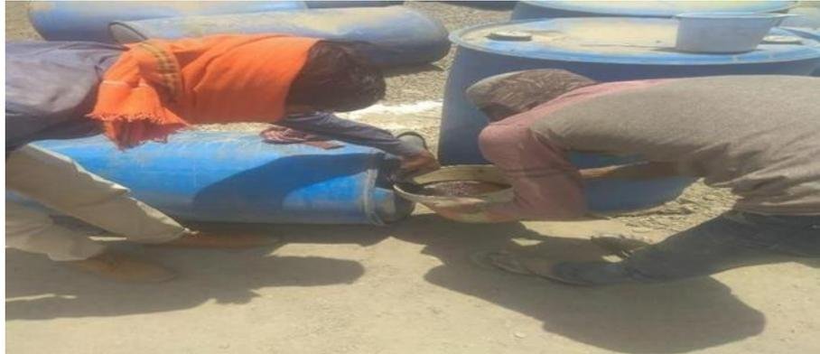
**Fig3.14- Sampling of Bitumen Emulsion from Stock Yard**
