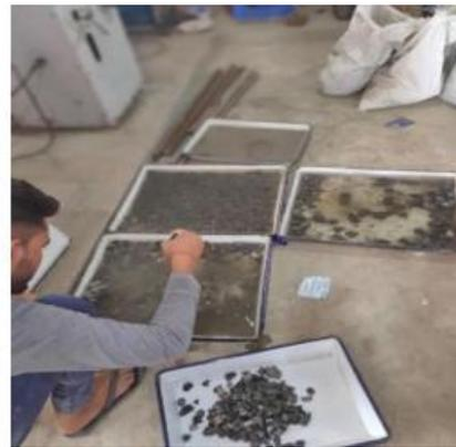
**Fig3.12-Different Size of Aggregates**
