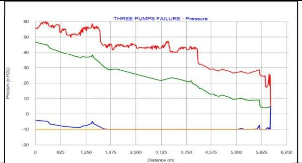
Fig.8: Pressure variation envelope plot without any surge protection throughout the rising main (Three Pumps Failure)
