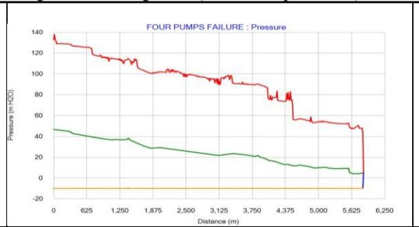
Fig.10: Pressure variation envelope plot without any surge protection throughout the rising main (Four Pumps Failure)
