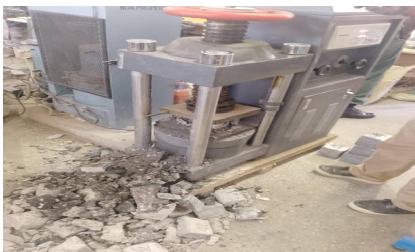
Fig 3.6 Crushing of cubes
