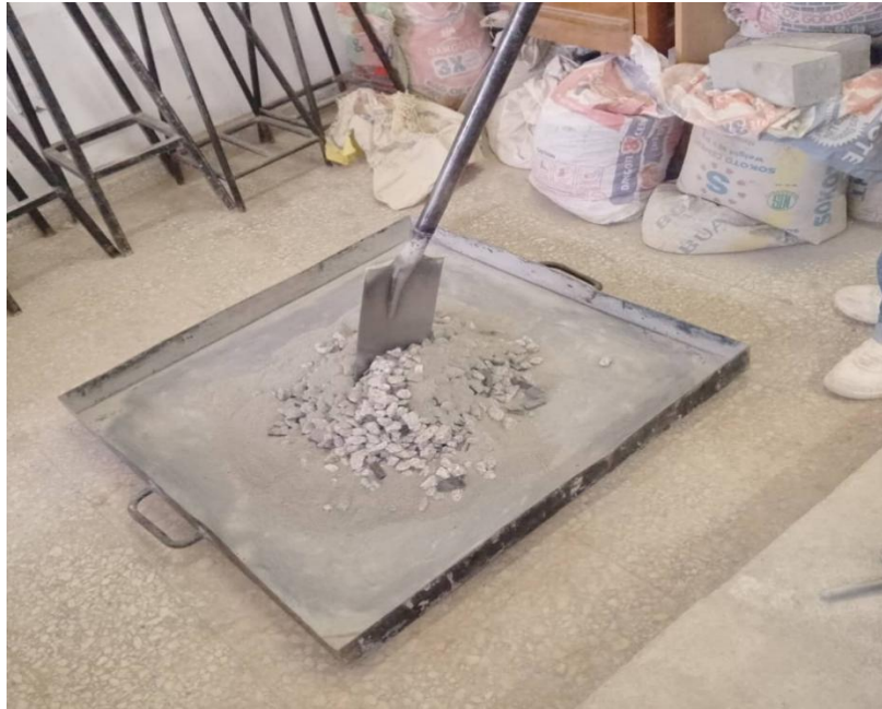
Fig 3.1 Mixture of Cement + ceramics, fine Aggregates and Coarse Aggregate + tyre
