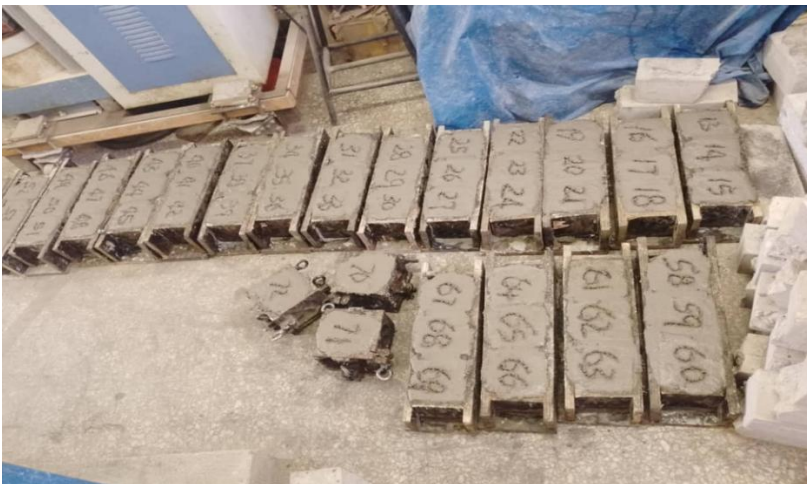
Fig 3.4 Concrete Cubes Before Demoulding
