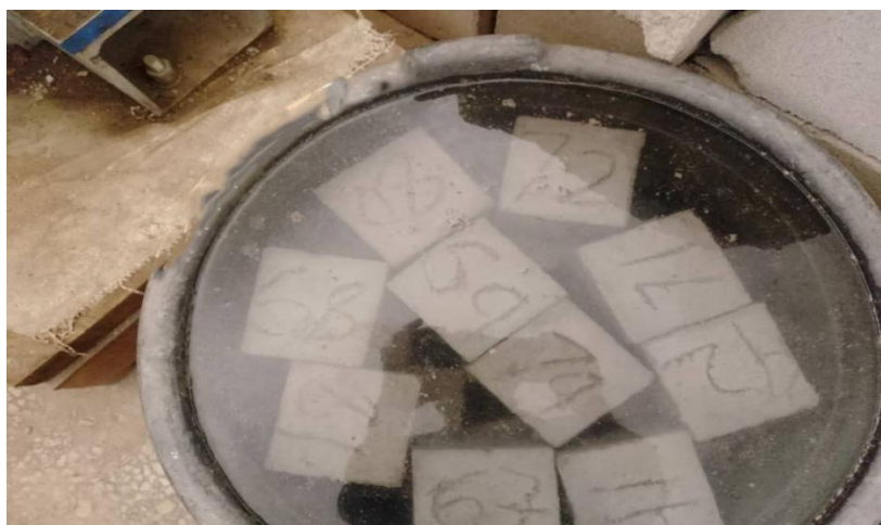
Fig 3.5 Curing of cubes
