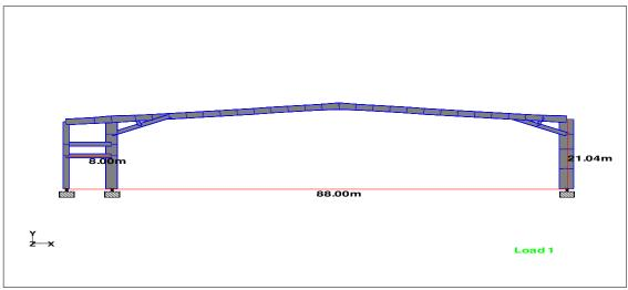
Figure 8- Long Span PEB Plane Frame
