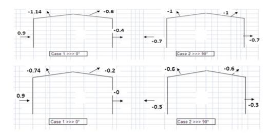
Figure 7- Wind Coefficients
