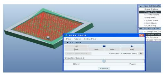
After completion of tool play path to check the required part shape is obtained or not checked by using NC check in Pro/E. it is illustrared in fig.2.6
