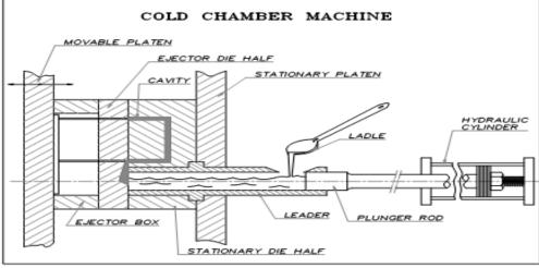
Fig. 1.2 Cold-Chamber Machine
