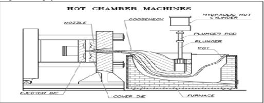
Fig. 1.1 Hot-Chamber Machine
