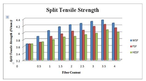
Fig. 5.2 Split Tensile Strength of concrete with percentage variation of Steel Fibress
