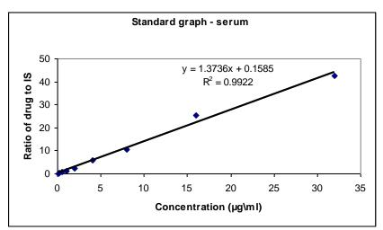
Fig. 3: Calibration curve was plotted against peak area ratio of RST & IS on Y-axis and Concentration on X-axis.
