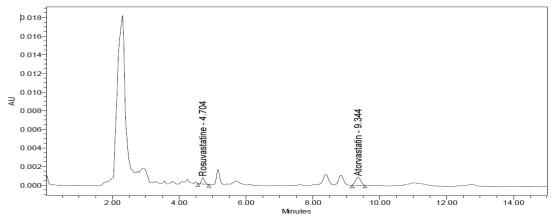
Fig. 2: Chromatograph with drug and internal standard eluted at their respective retention times.
